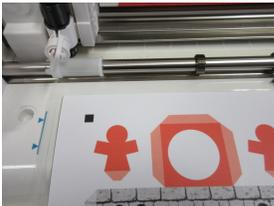
**Cameo instructions:** Align the left edge of the cut mat to the blue guide line on the left side of the feed area.
